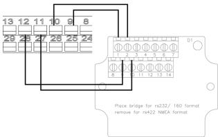
Recommended cable: shielded 2x2x0,75mm2 twisted pair
