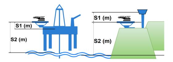
Always use the height of the location of the barometric sensor itself, even if a pressure head (OMC-509) is used. The location of the pressure head is irrelevant for the sensor height! The sensor is preferable build in the same housing as the OMC-183-ML.
