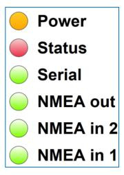
If you experience difficulties connecting with the device; Check if the LED's are blinking, Check the wiring of the Tx/Rx or A/B wires; Check the data settings of your COM port.
